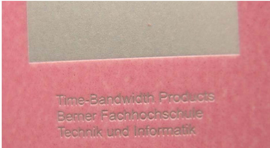
Precise selective ablation of layers on polymer substrate
