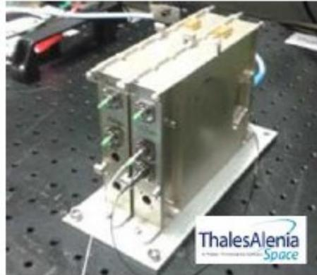
Figure 4-21: Photonic Frequency Converter
