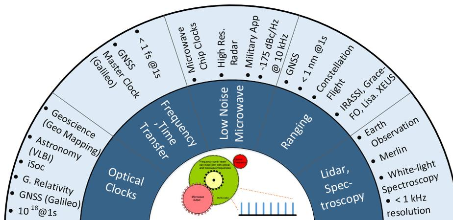
Figure 4-8: Frequency comb space applications.
