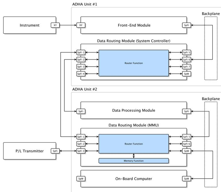
Figure 4-16: Two ADHA unit implementation of a satellite avionic architecture.
