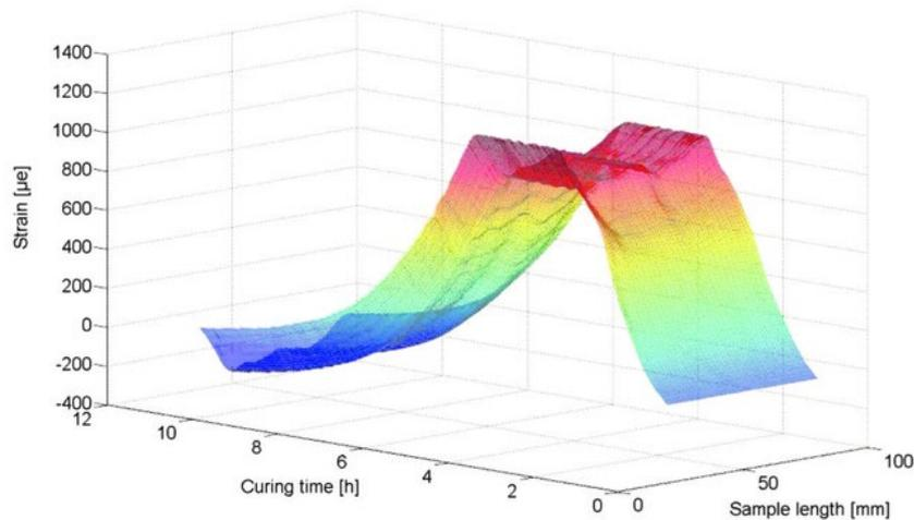
Figure 4-31: Strain distribution in a composite panel measured using an embedded optical fiber.
