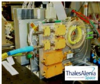
Figure 4-22: Photonic Router/Wavelength Selective Switch
