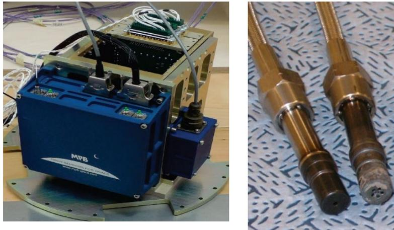
Figure 4-28: Right - High temperature experiment on ROTEX. Left - High temperature fiber optic pressure sensor from Oxensis after Thermal testing.
