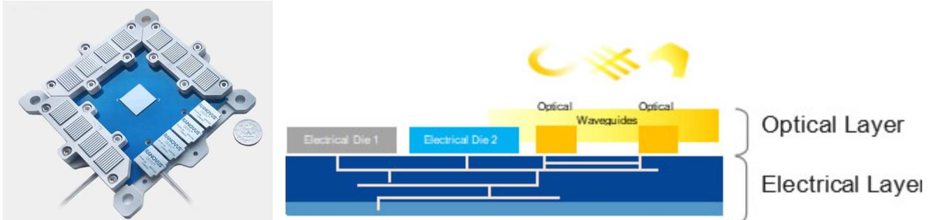
Figure 4-7: Transceiver Chiplets by RANOVUS and Interposer concept by POET technologies for >100 Gbps transmission.
