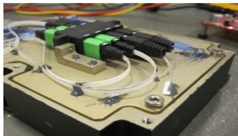
Figure 4-19: Hermod IOD on board PROBA V.
