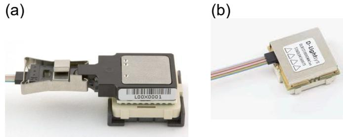
Figure 4-15: Parallel transceiver packages from a) Smiths Interconnect, b) RADIALL (ex D-lightsys).
