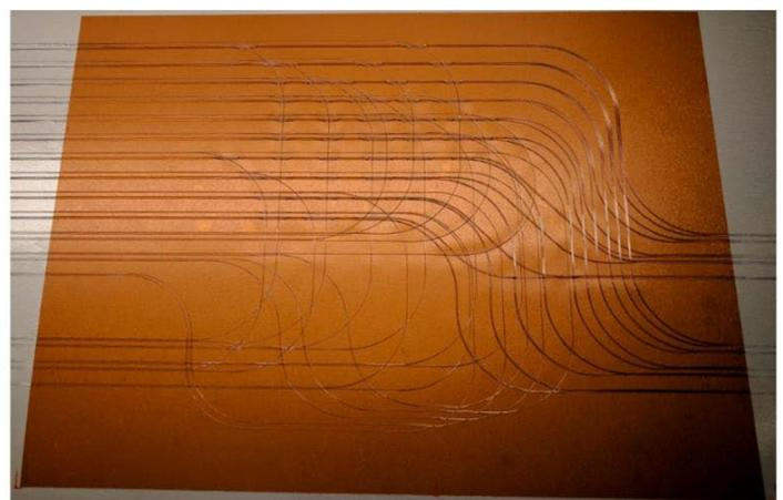
Figure 4-14: Fiber Optic Routing Assembly [RD-FOFRA].
