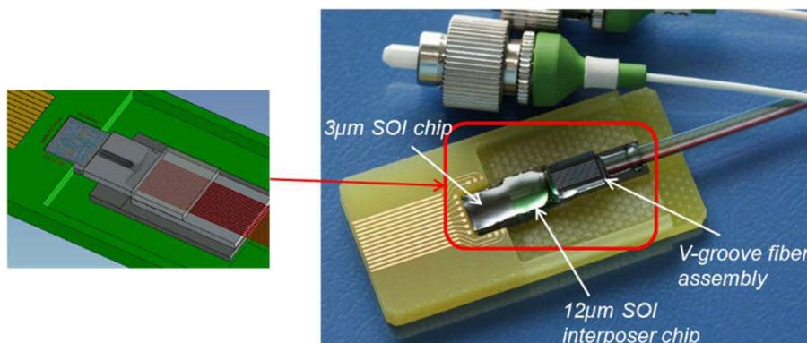
Figure 4-23: VTT Standard SMF to SOI PIC package design.
