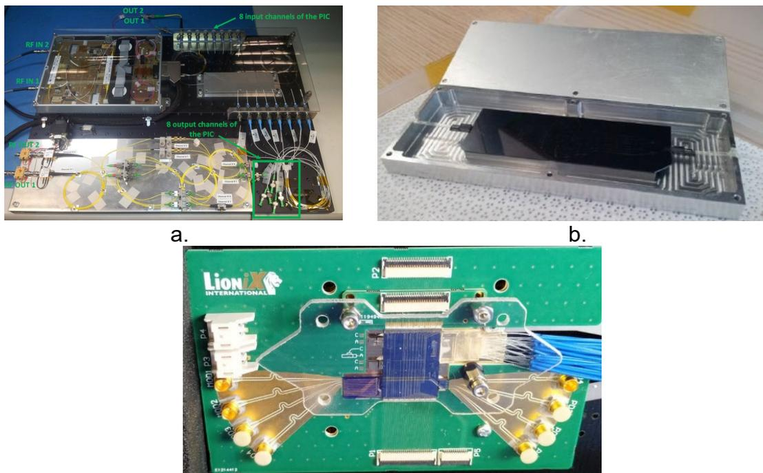
Figure 4-26: Microphotonic integrated Optical BFN fully assembled. Figures a) and b) show a passive Silicon based Butler matrix type BFN made by DAS Photonics. Figure c) shows a BFN based on a hybrid InP active part combined with a passive Silicon Nitride made by LIONIX.
