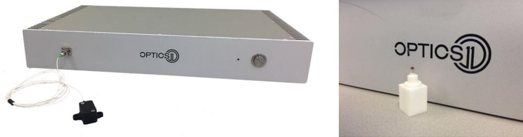
Figure 4-32: Optics 1 optical sensor interrogator (left) and 3-axis accelerometer prototype (right).
