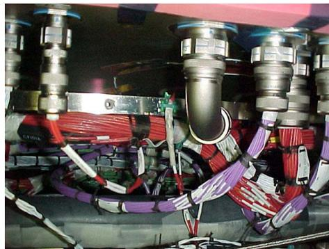
Figure 4-10: Optical fibers on the ISS (purple colour).
