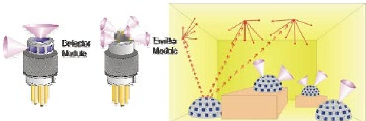
Figure 4-27: Optical Antennas for diffused infrared transmission.
