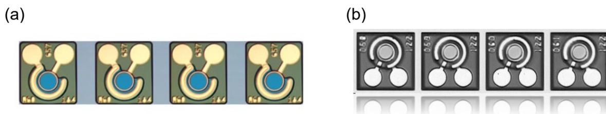
Figure 4-9: PIN diode arrays from a) Coherent, and b) Trumpf.
