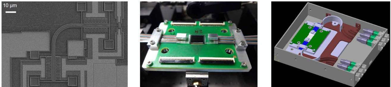
Figure 4-24: EPFL optical switch, silicon design, packaged PIC and equipment design.
