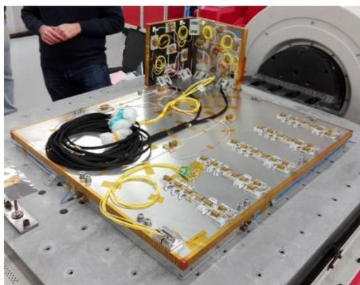
*Figure 4-29: HPS built photonicly wired panel undergoing vibration testing.*
