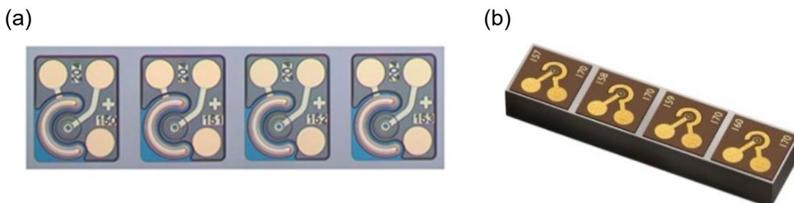
Figure 4-5: VCSEL arrays from a) COHERENT (ex II-VI Laser Enterprise), and b) TRUMPF.
