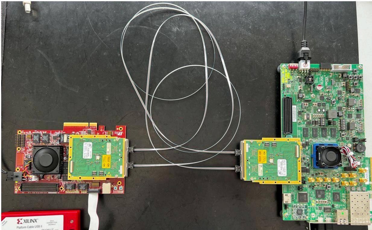
Figure 4-17: An 8 port SpaceFibre demonstrator implementation on a Xilinx FPGA over fiber optic transceivers.
