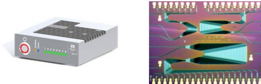
Figure 4-30: Photon First (NL) Microphotonic FBG Interrogator based on InP Photonic Integrated Chip.
