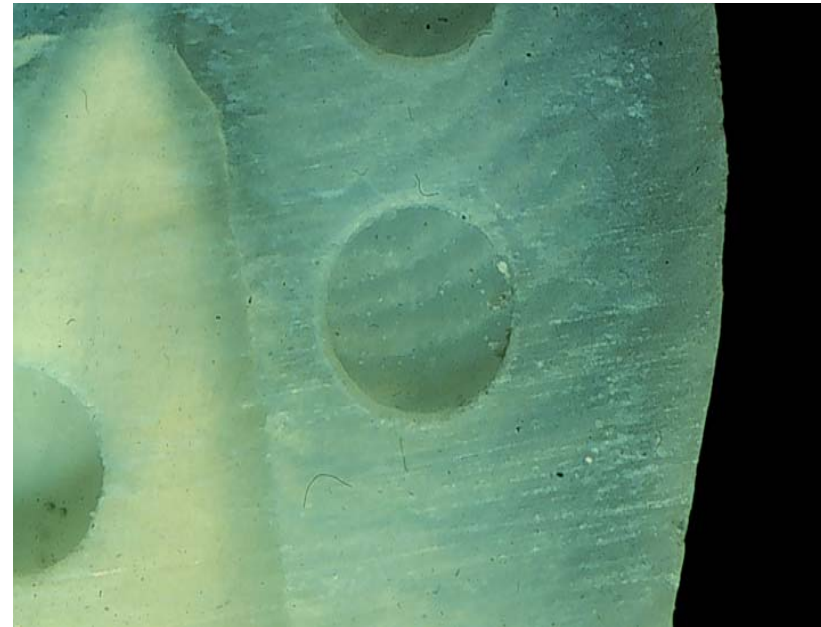
193 nm Excimer-Laser <1 \mu\text{m} pro Puls
