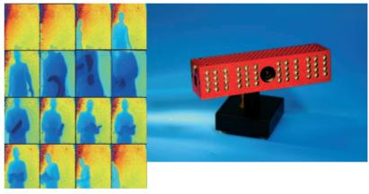
Fig. 3.5.6 Left: A few scenes out of a 3D movie acquired with an optical time-of-flight range camera. The distance images are color-encoded (dark blue = 10 cm; red = 750 cm); right: Miniaturized optical time-of-flight range camera with millimeter resolution, based on a custom CCD/CMOS image sensor with smart pixels © CSEM
