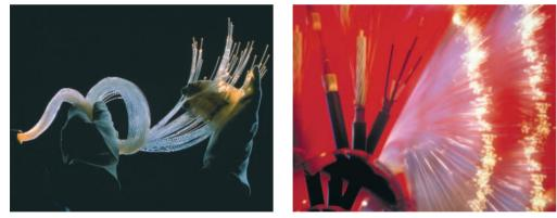
Fig. 3.1.5 Light transmission through optical fibres will enable transmission capacities per carrier in the 100 Tbps range by 2015 © left: Telekom; right: France Telecom
