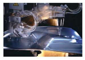
Fig. 3.2.1 Laser processing system for cutting and welding © Trumpf
