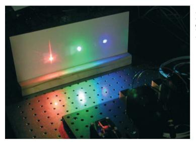
Fig. 3.4.16 Laser devices for projection applications © Osram Opto Semiconductors For these purposes, an entirely new core technology of powerful, efficient and compact laser sources in the visible range as well as novel system architectures are necessary.
