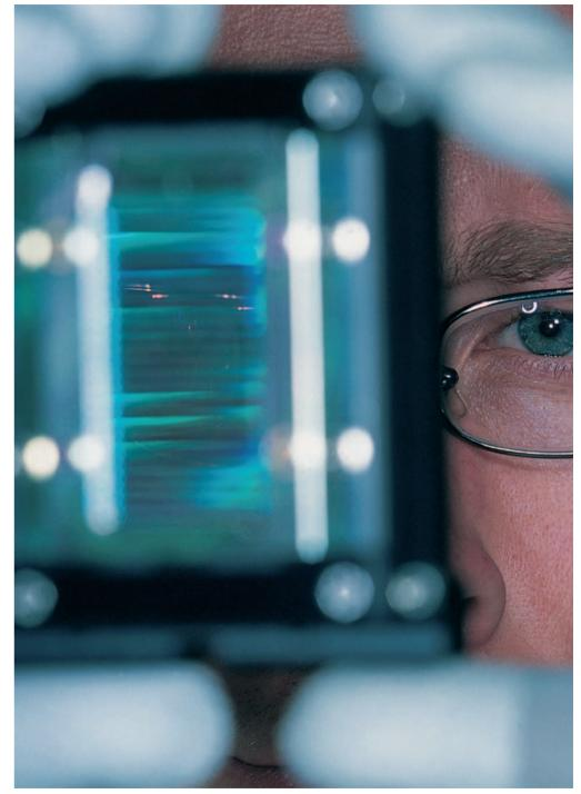
Fig. 3.6.7 Diode lasers are the most efficient artifical light sources existing. Due to their high efficiency and long service life, they have proved a success in many applications. The extremely compact diode lasers are increasingly gaining importance as light sources for direct treatment in industry and medicine and as highly efficient pumping sources in solid state lasers © Jenoptik
