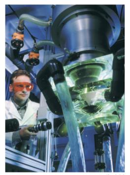
Fig. 3.5.3 Analysis of air and fuel flows within ducting components through optical laser methods © Bosch
