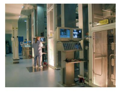
Fig. 3.6.2 Top floor of the fiber draw tower where the preform is heated up to approximately 2000 ℃ in order to draw the fiber © OFS Fitel
