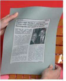
Fig. 3.4.11 Flexible active matrix e-paper SVGA display printed at Plastic Logic's Prototype Line in Cambridge, UK © Plastic Logic Limited An example would be a rollable display with a wireless interconnection for new content, such as e-newspaper displays.
