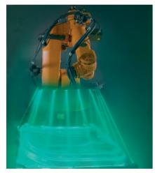
Fig. 3.2.4 Laser remote welding © Kuka
