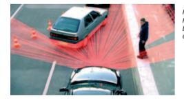
Fig. 3.5.7 Pedestrian and traffic perception by a laser scanner in a vehicle © IBFO
