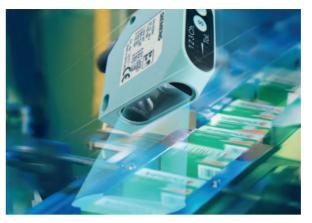
Fig. 3.5.4 Quality control with white light LED detectors © Siemens
