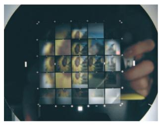
Fig. 3.6.3 Wafer with 5 x 5 ultra-thin (< 0.3 mm) artificial compound eye objectives (before dicing) imaging a picture of sunflowers © Fraunhofer IOF
