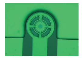
Fig. 3.6.6 Microscope image of a high speed VCSEL for data communication applications © Chalmers University of Technology
