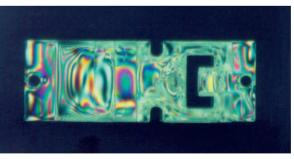
Fig. 3.5.5 Mechanical stress analysis of complicated objects can be carried out by employing the optical birefringence of polymers, showing up as color patterns © CSEM
