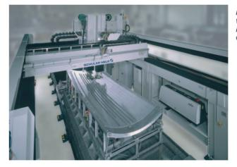
Fig 3.2.2 Welding of stringer profiles in aircraft construction © Schuler Held Lasertechnik
