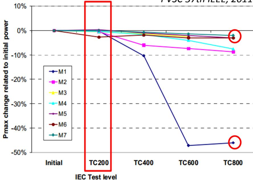
Thermal Cycling test (IEC 61215):
