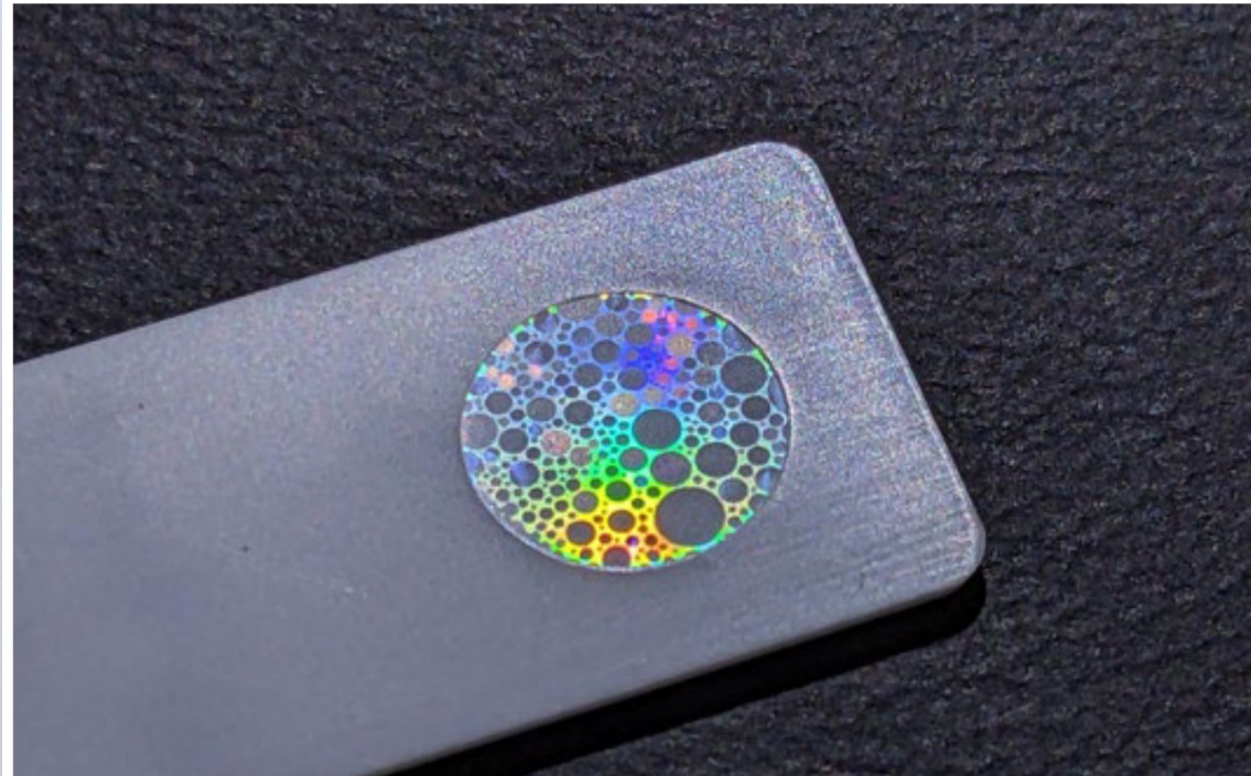
Fig. 1 Optimising the Ceramic Injection Moulding process with variotherm technology delivers improvements in process stability and quality. In relation to the manufacture of holographic structures such as this, significant advances in quality and process capability are achieved (Courtesy iRAP Institute, HEIA-FR/HES-SO, Morphotonix)
