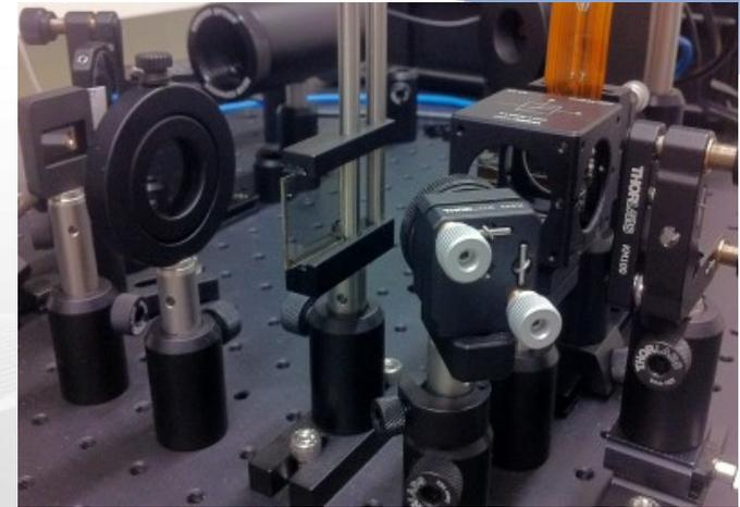
*High-speed interferometric measurement system*
