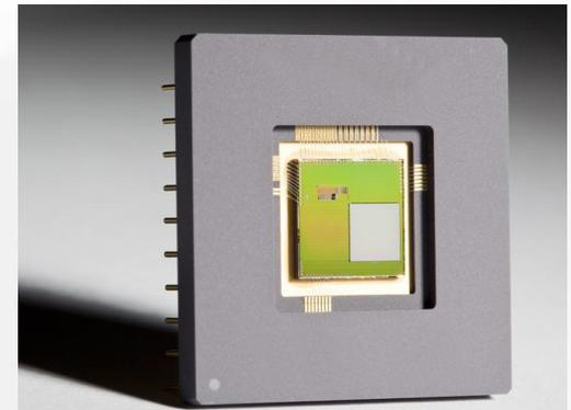
CMOS-based 240x200 piston-type MEMS, courtesy of Fraunhofer IPMS
