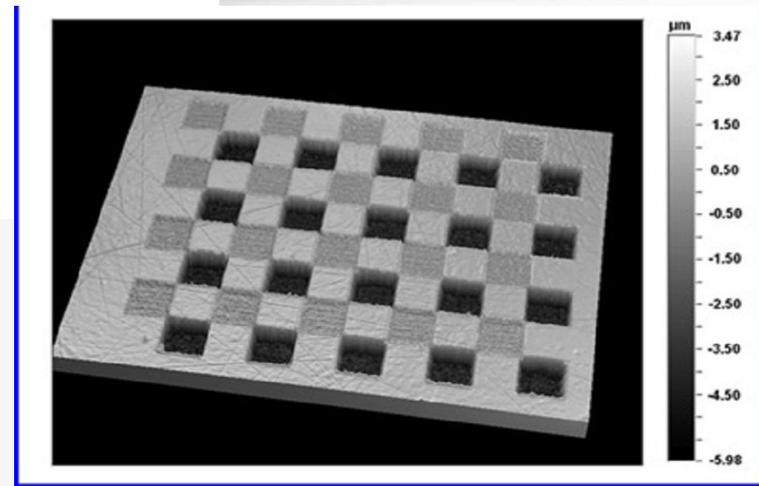
Images courtesy University of Liverpool. Z. Kuang, et al., Fast parallel diffractive multi-beam femtosecond laser surface micro-structuring, Applied Surface Science (2009)
