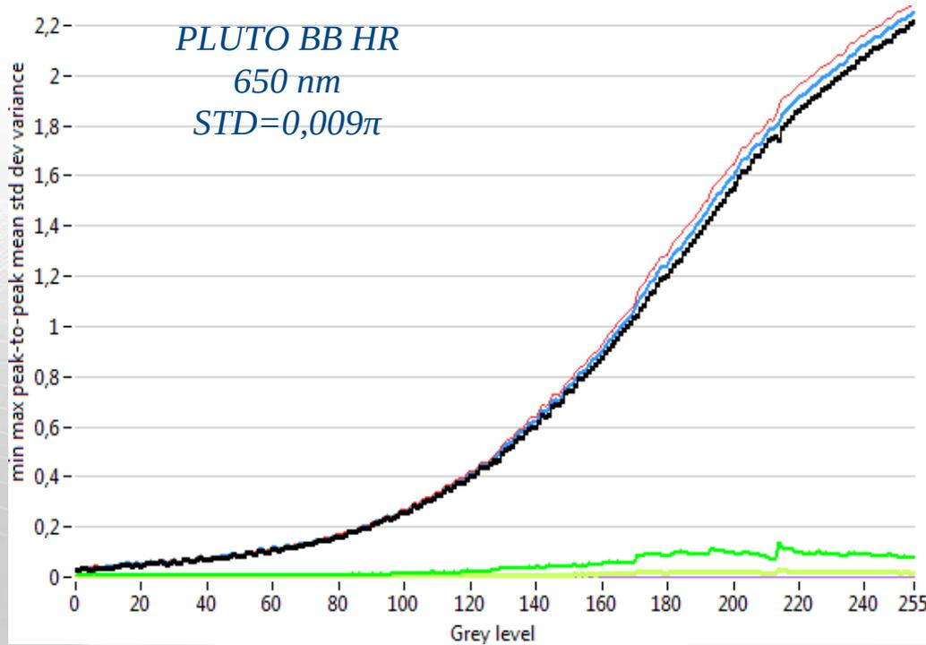
*Signal/Modulation properties vs. addressed „grey level“, measured with interferometric system. Red - max. phase, black – min. phase, blue – mean phase, green – standard deviation, yellow - variance*
