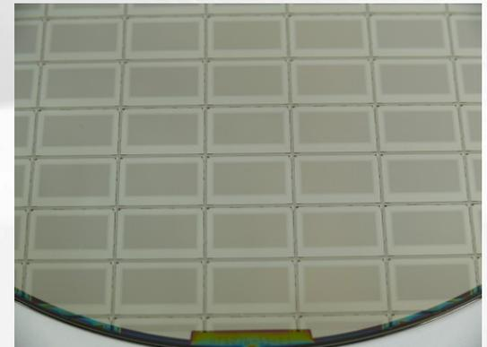
*0.25 micron process 8" CMOS wafer - 0.7" HD LCOS*
