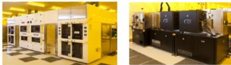
S2S and R2R deposition tools and laser cutting and finishing
