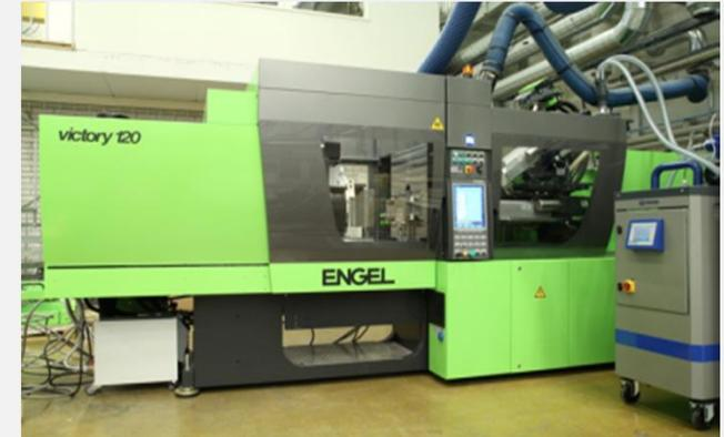
ENGEL injection moulding machine with R2R feeder
