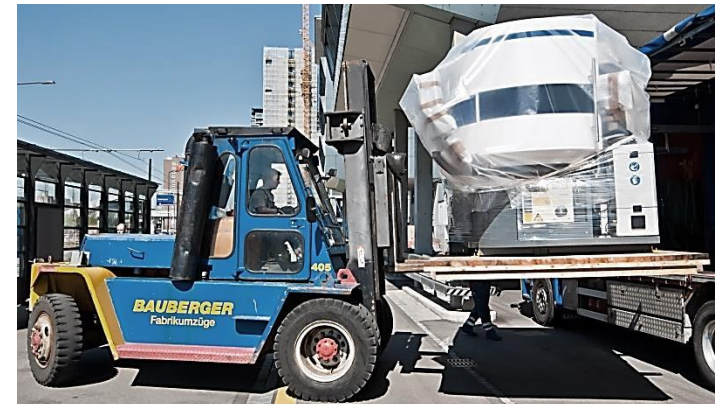
Delivery of a machine with installed ultrashort pulsed laser system. Shock events up to 10g when handling system.
