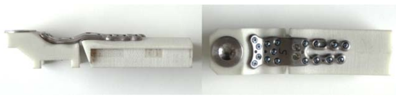
Fatigue test: Comparison between commercially machined plates and SLM plates.
