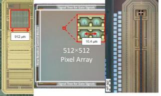
Fig. 1. Micrographs of Piccolo, a  $32 \times 32$  SPAD array with photosensitive area on the top section, highlighted in red (left) [41,42] – see also Fig. 8 (center); SwissSPAD2 512 × 512, a gated SPAD imager with 4 pixels shown in the inset (center, featuring round SPAD active areas in this case) [45]; Detail of LinoSPAD2, a 512 × 1 linear SPAD array with top alignment cross integrated in the metal stack (right).
