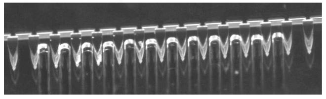
12<sup>er</sup> fiber ribbon fully inserted against the reflecting element
