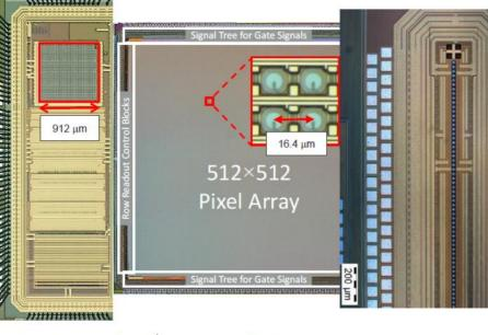
**Fig. 1.** Micrographs of Piccolo, a  $32 \times 32$  SPAD array with photosensitive area on the top section, highlighted in red (left) [41,42] – see also Fig. 8 (center); SwissSPAD2 512 × 512, a gated SPAD imager with 4 pixels shown in the inset (center, featuring round SPAD active areas in this case) [45]; Detail of LinoSPAD2, a 512 × 1 linear SPAD array with top alignment cross integrated in the metal stack (right).
