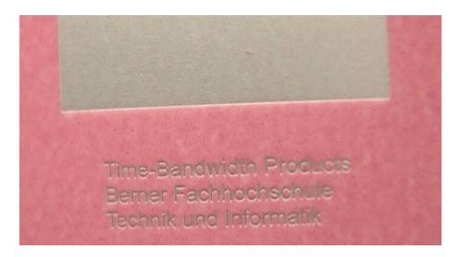
Precise selective ablation of layers on polymer substrate
