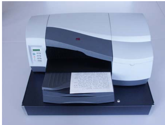
Prototype of home printer with blue light LED curing system
