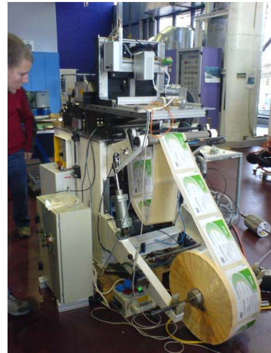
Industry-version of Braille printer with UV curing system
