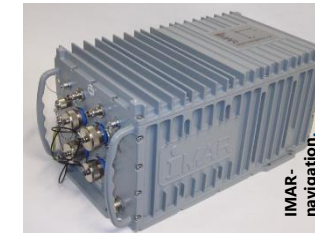
Fiber-optic Gyro (FOG) Sagnac interference
