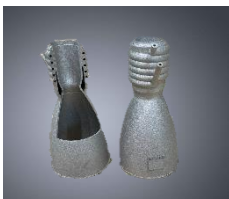
AM – Satellite thrusters Material: C103 (Niobium) EXHIBITION SAMPLE
