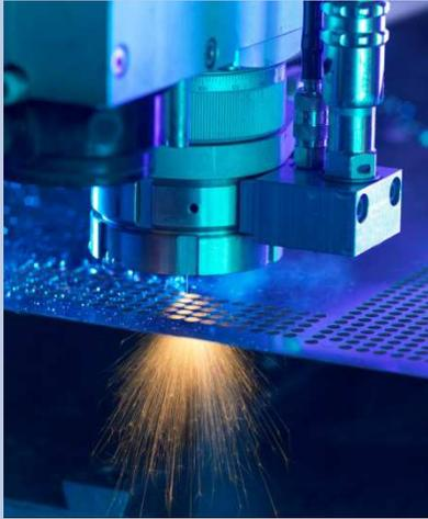
watch parts cut with Laser MicroJet®
