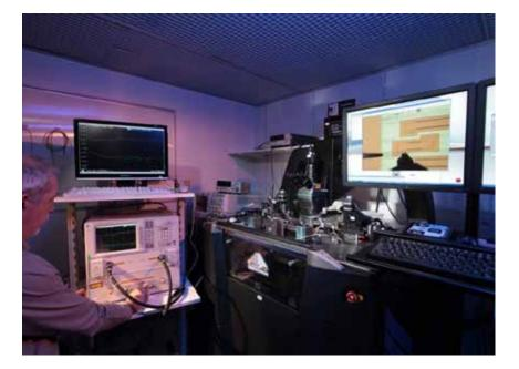
Wafer-level probe testing on 200/300 mm silicon wafers. © CEA-Leti with developments in new optical elements, such as stacked micro-optics technologies and freeform optical surfaces. The emergence of laserassisted manufacturing processes and of printing technology for additive deposition of functional materials offers further potential for enhancing competitiveness.
