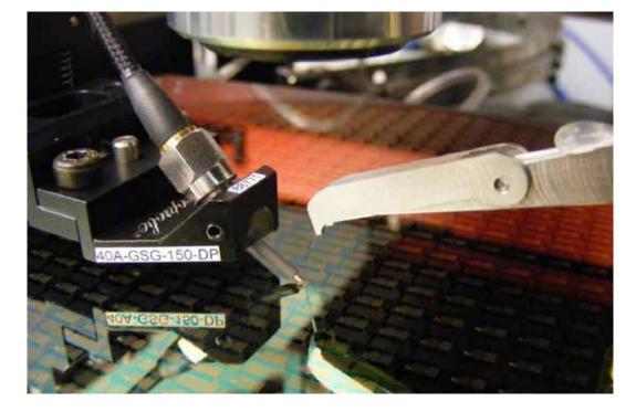
High frequency wafer level testing of germanium photodiodes on silicon. © CEA-Leti
