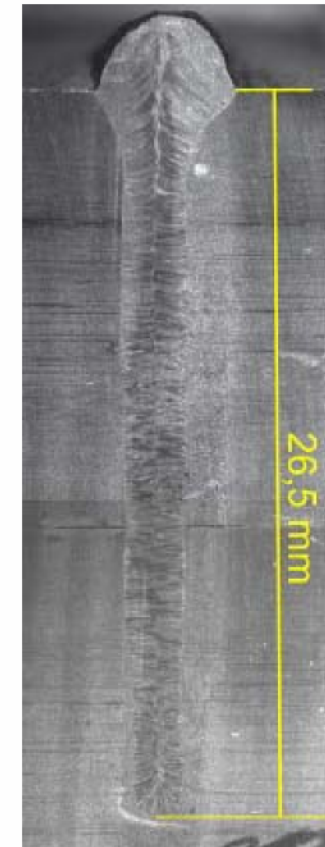
Overlap joint 2x 15 mm Stainless steel 1.4301
