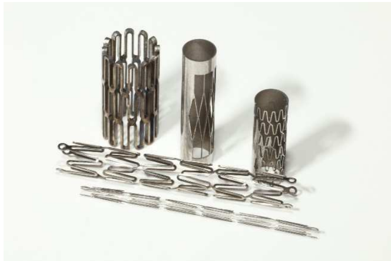
Stent cutting with ultrafast laser
