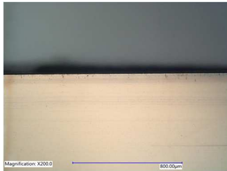
Ablation/cutting of ultra-hard materials
