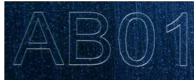
Outline Marking in Glass and Sapphire
