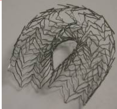
Cutting Nitinol Coronary Stents - 100W
