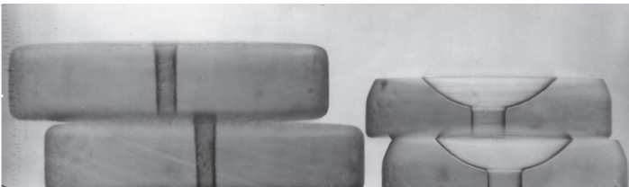
Fig. 23: Nd:YAG drilled holes (diam. 50\ \mu\text{m} ) in 0.3\ \text{mm} thick ruby discs (diam. 10\ \text{mm} ) and finished watch bearings [100].
