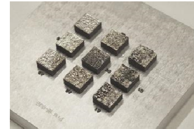
Al 6061 by SLM (3D System – CEA Tech)
