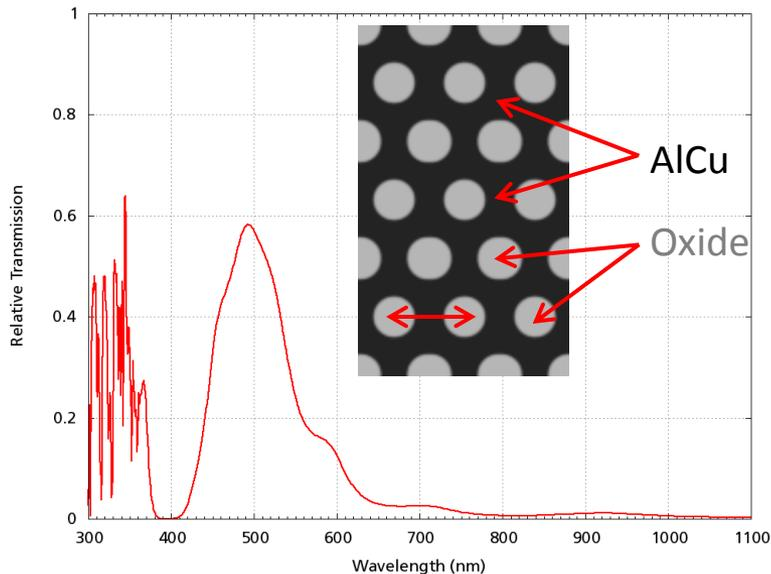
Spectral transmission of a hole array
