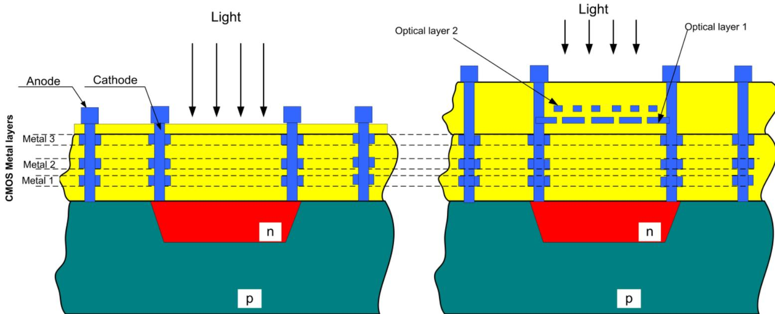
Conventional CMOS photodiode
