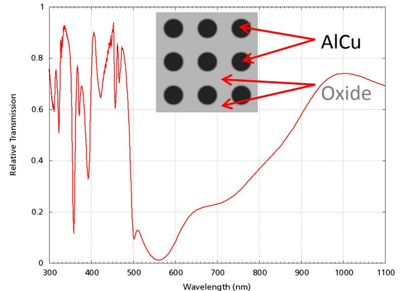
Spectral transmission of an island array
