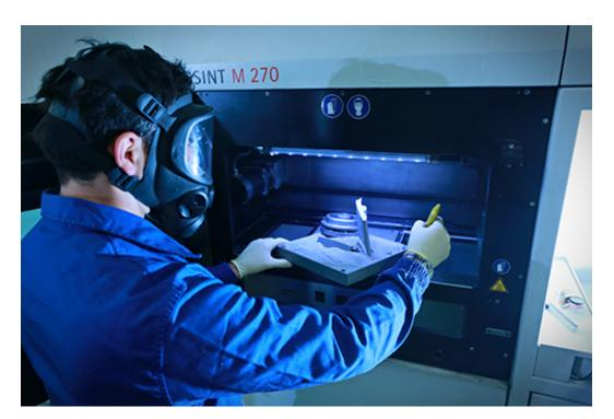
Post processing of additively manufactured parts
