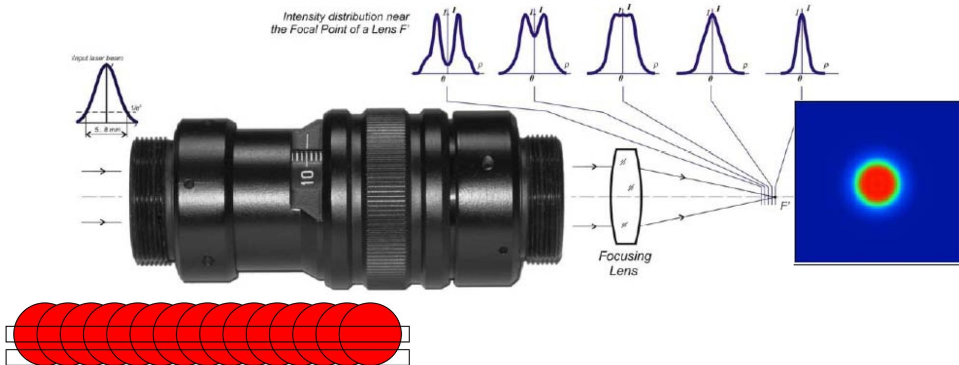
When a round top hat beam moves over a surface more energy per area is deposited in the center of the line than at the borders.
