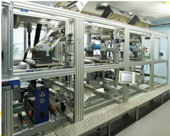
R2R printing with pilot machine
