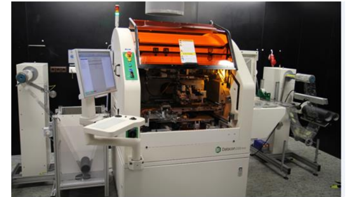
R2R assembly pilot machine
