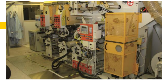
PICO – in-air roll-to-roll pilot line
