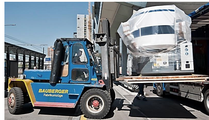
Fig. 2: Delivery of a machine with installed ultrashort pulsed laser system. Shock events up to 10g when handling system.
