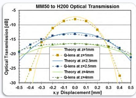
Results of Q-lens (r=780 μm) with MM as input fiber at different z-distances in comparison to simulations
