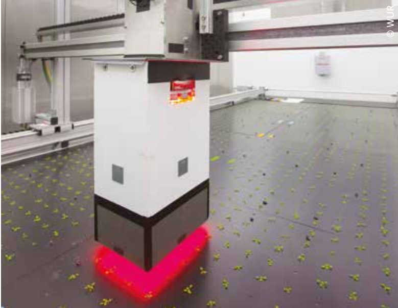
Right: Phenovator at Wageningen University & Research. Automated data collection of the performance of plants (phenotyping) in a growth room using Chlorophyll Fluorescence Imaging. By using active LED lighting the photosynthetic capabilities of a plant is measured.
