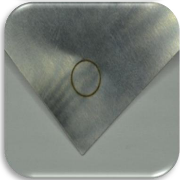
Bottom weld view full penetration
