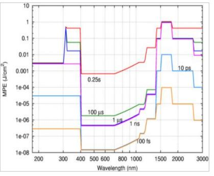
MPE as energy density versus wavelength for various exposure times (pulse durations)
