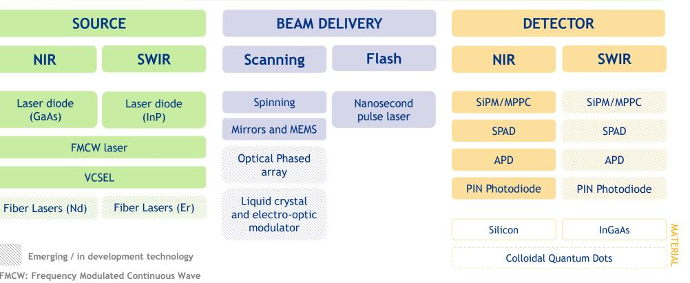
FMCW: Frequency Modulated Continuous Wave VCSEL: (Vertical-cavity surface-emitting laser) MEMS: MicroElectro-Mechanical Mirrors SiPM/MPPC: Silicon Photomultipliers/MultiPixel Photon Counters SPAD: Single-Photon Avalanche Diode APD: Avalanche PhotoDiode
