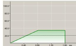
Pulse shaping may not be required but has been shown to yield improved results for micro welding.
