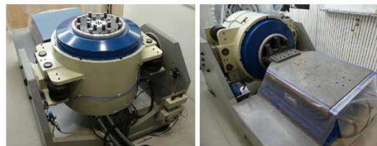
Ling 2016 shaker, 89 kN, vertical orientation
