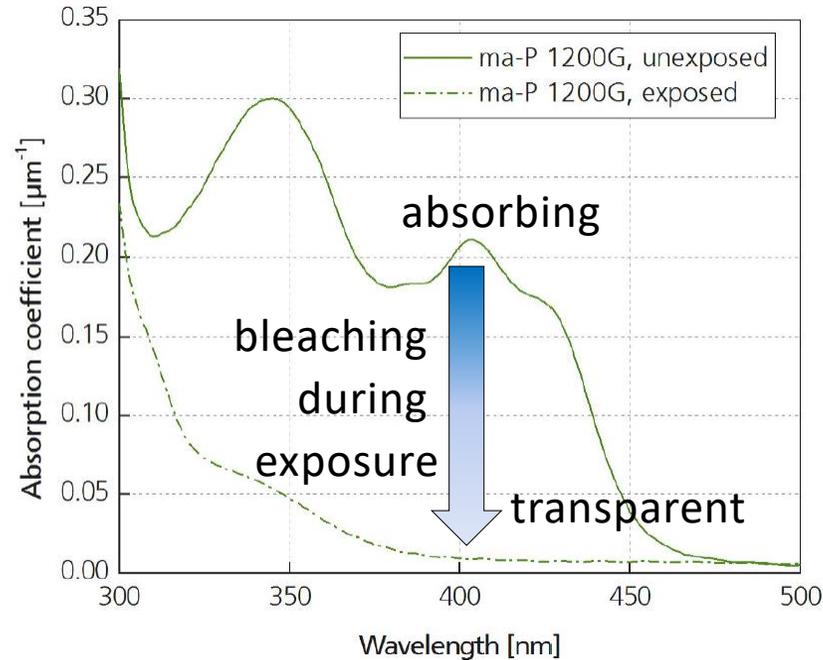
UV/vis absorption spectra of unexposed and exposed ma-P 1200G
