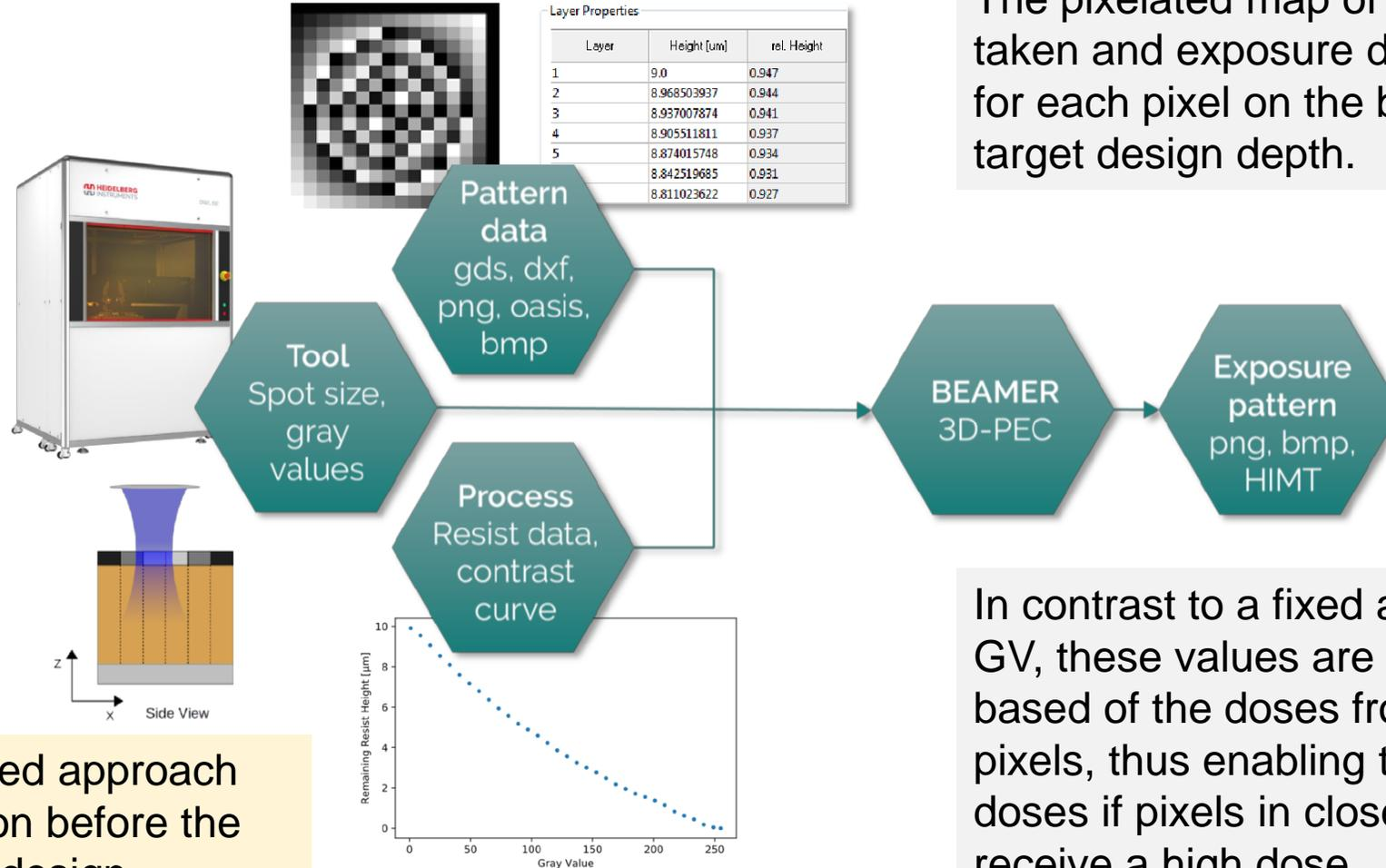
The pixelated map of a layout is taken and exposure doses assigned for each pixel on the basis of the target design depth.
