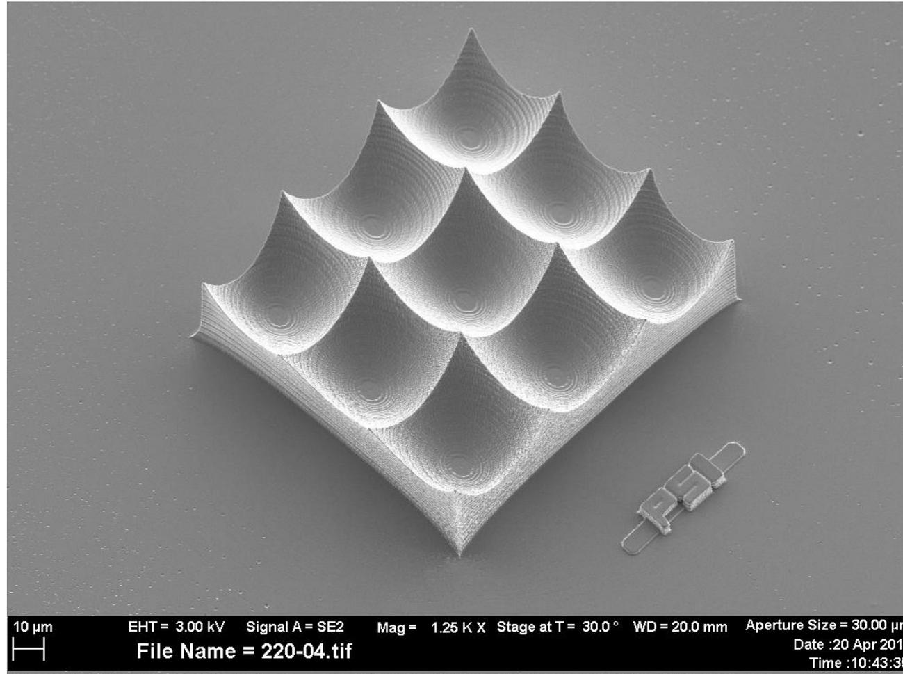
**Test structure:** Micro-lens array (3x3) concave 50 µm x 50 µm x 50 µm (each)
