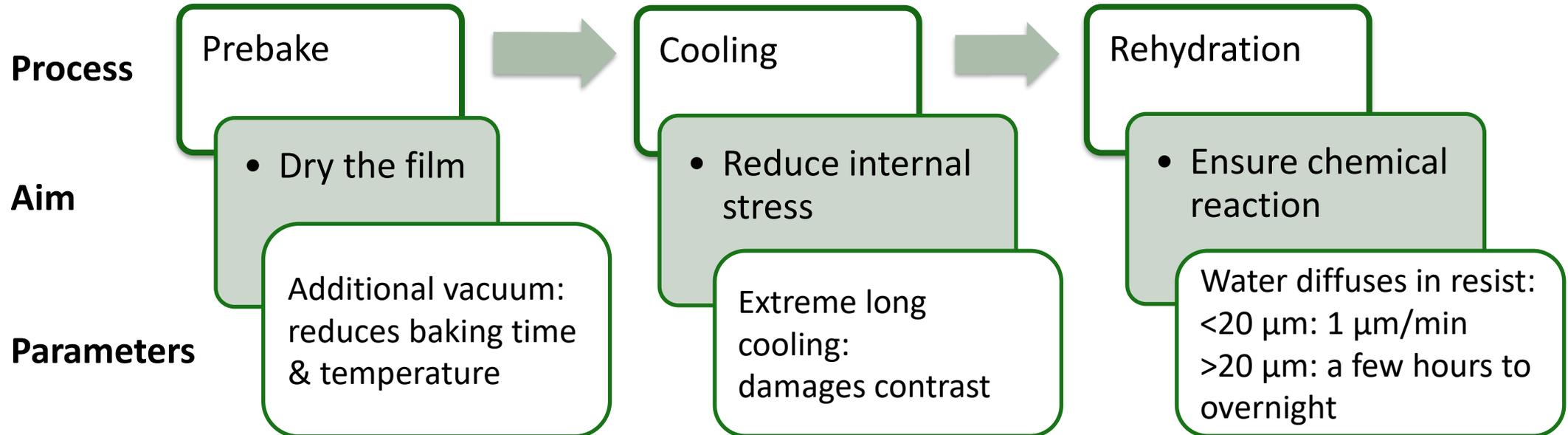
Working thickness up to 60 μm; more critical for thickness >20 μm
