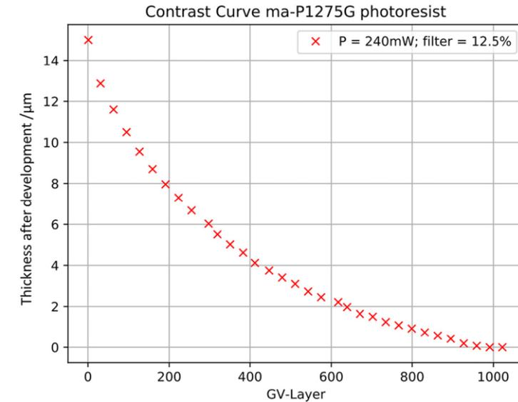
Contrast curve (in linear scale) of ma-P 1275G (33 measurements for 32 exposure doses) from zero dose at 15 μm height down to dose-to-clear at 0 μm (thickness after development)
