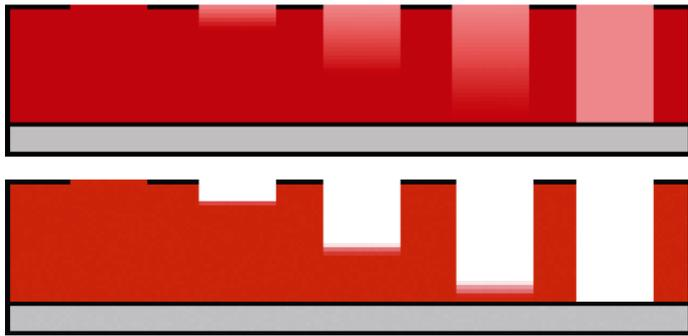
Top: Grayscale exposure of thicker resist films (FT ≥ 5 μm); Bottom: resist pattern after development.
