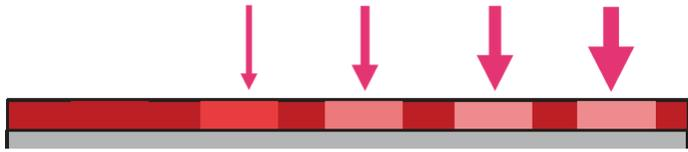
Figure 3: Grayscale exposure of thin film resist (FT ≤ 5 μm)
