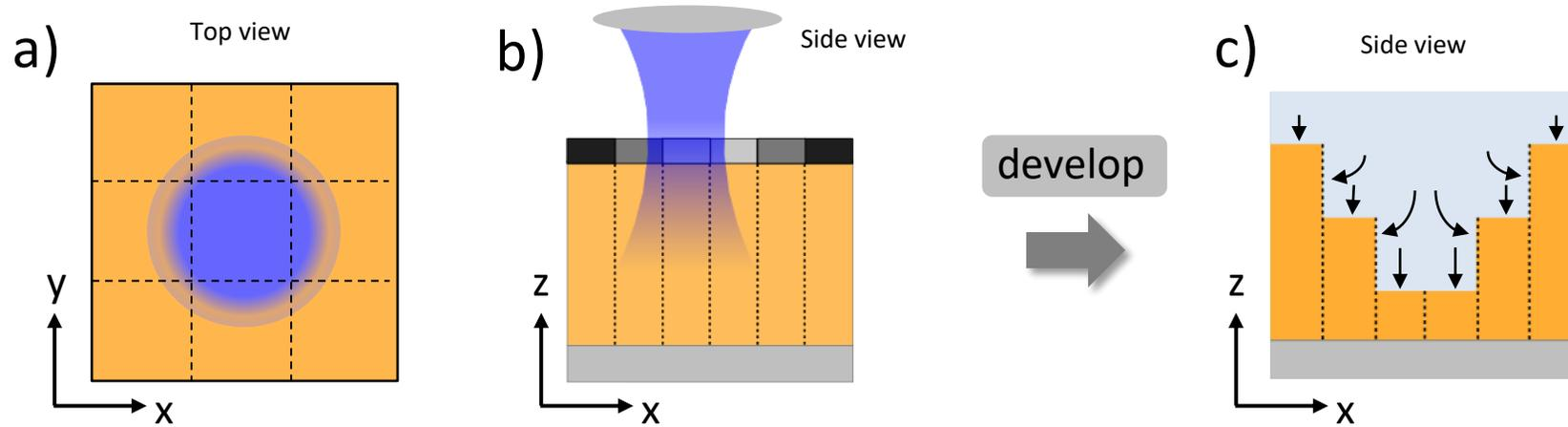
Progression of development fronts into positive resist (3D resist simulation in LAB)
