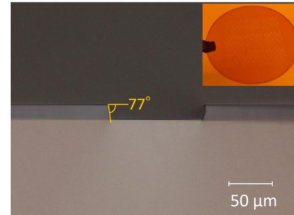
→ Side wall angle of ma-P1275G and mr-DWL40 for 20 μm thickness are almost similar (78° )
