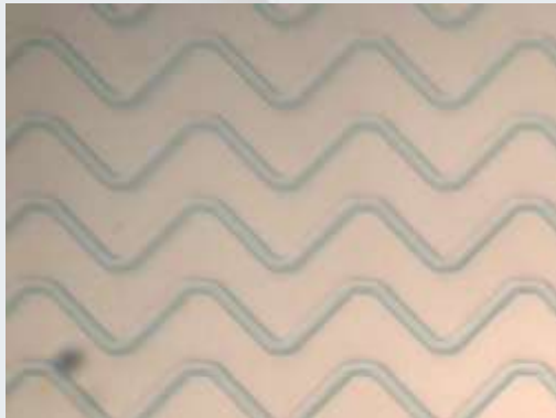
Patterning - 10 micron wide tracks on 70 micron pitch
