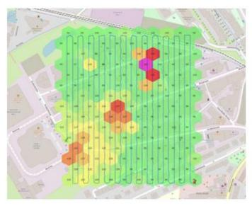
Within few minutes, operators can define the UAS flight path for upcoming missions. Depending on the mission type, and the expected amount of radioactivity, an operator will choose an according altitude above ground, flight speed, and flight path overlap.
