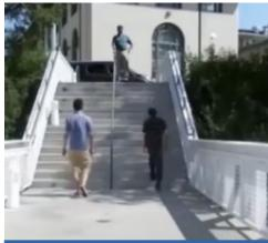
Scene with strong ambient light. The illumination of the TOF camera competes with sunlight - ranging is very challenging. In addition, the person with black clothes is hardly visible.
