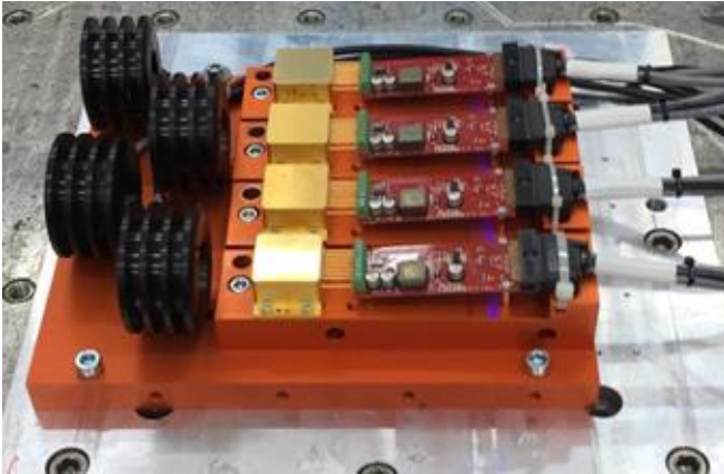
Vibration profile 0.04g²/Hz (MIL-STD 810F)
