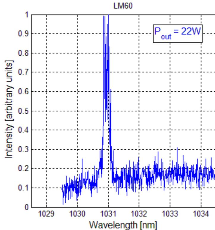
→ Wavelength selection + stabilization with intra-cavity GWS
