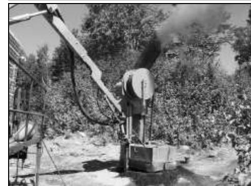
spallation drilling plant in the field
