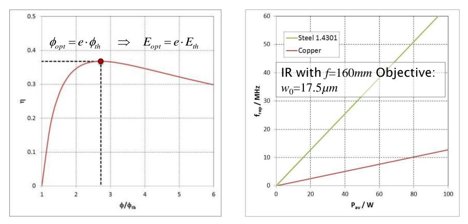
Already at low average powers high repetition rates are demanded to work at the optimum point with maximum efficiency.
