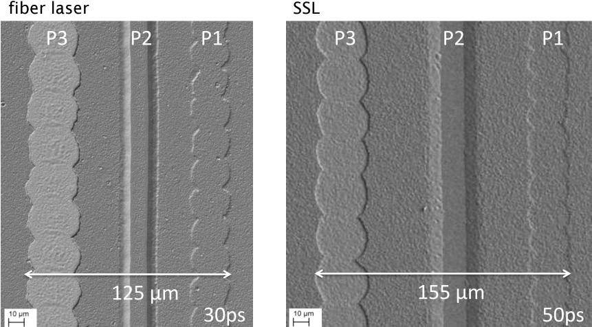
SEM image of complete module interconnect. Similar scribe quality is realized with SSL and fiber laser.
