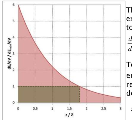
The deposited energy per unit volume exponentially drops with the distance z to the surface.
