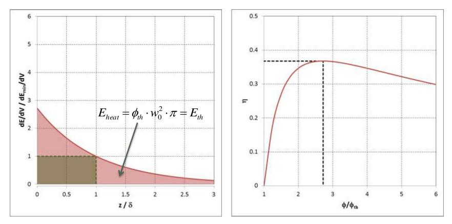
The efficiency  $\eta$  shows a maximum with:  $\eta = 1/e = 36.8\%$  and  $\phi = e \cdot \phi_{th}$ The ablation depth and volume per pulse then read:  $z_{abl} = \delta$ The deposited energy is independent of the pulse energy
